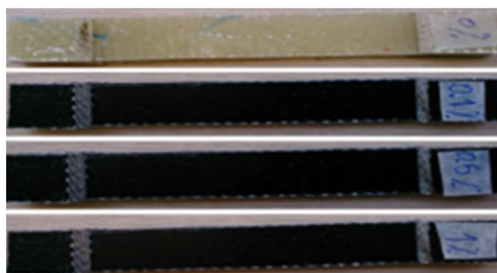
Fig.3 Typical of tensile test specimens hybrid nanocomposite
