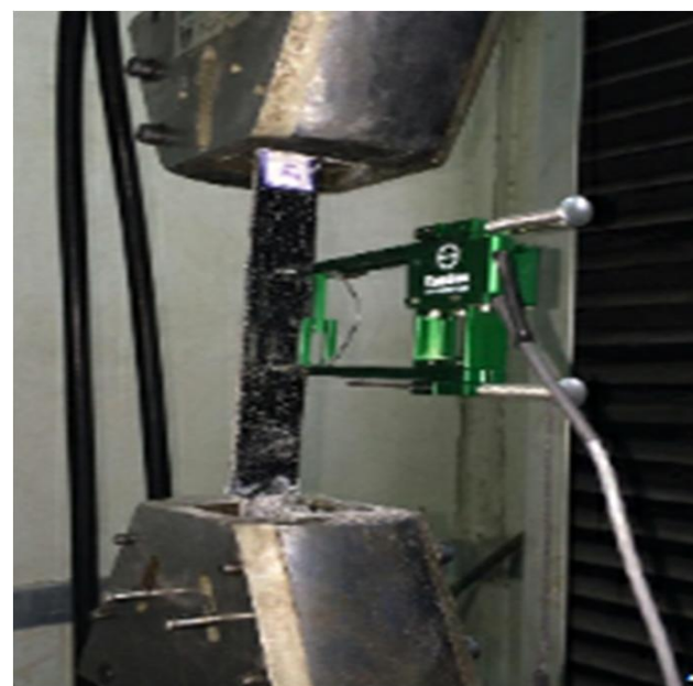
Fig. 5 Composite specimen under tension
