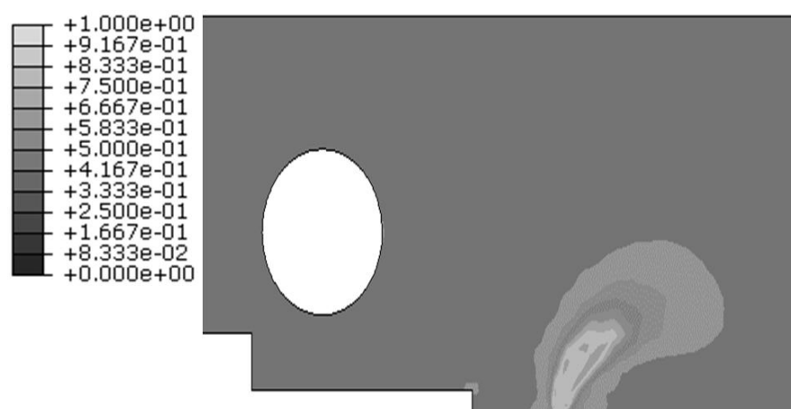
Fig. 15 Damage distribution ahead of P91 CT specimen crack tip after exposing to 10000 hours of creep condition at 650C and 3000N load
