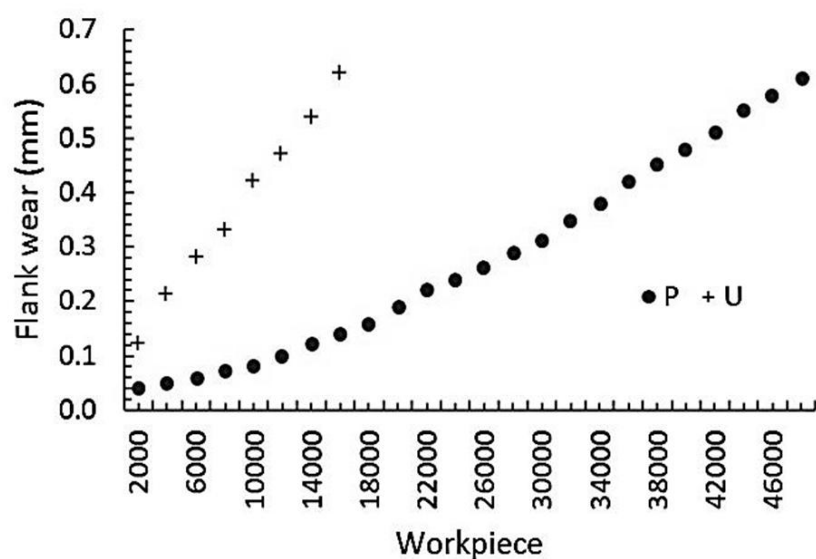
Fig. 8 Comparing flank wear of two drills according to drilled workpiece
