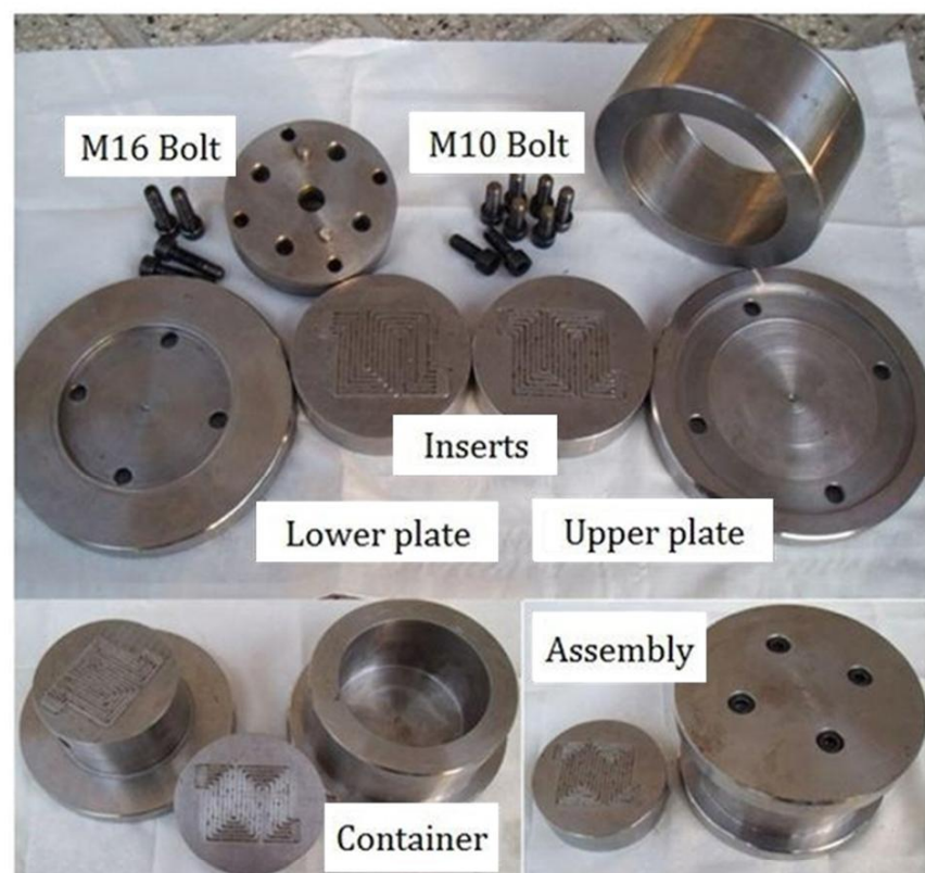
Fig. 11 Components of die in separate and assembled view
