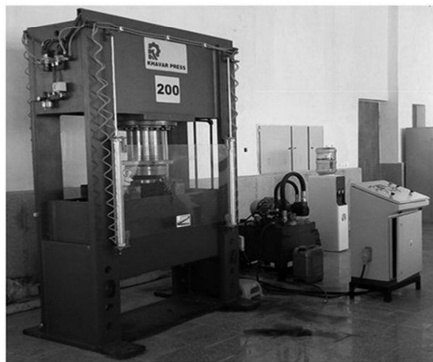
Fig. 12 Applied hydraulic stamping device for acting force on the die with capacity of 200 ton
