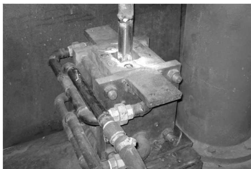
Fig. 2 A view of the ESR process
