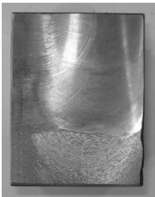
Fig. 3 the produced FGS ingot
