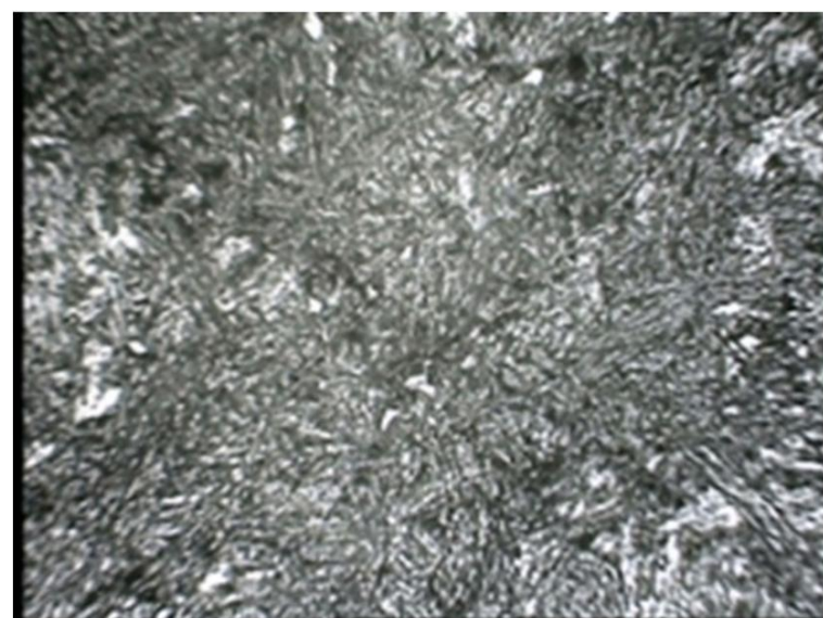
Fig. 5 The micro structure of the bainite phase
