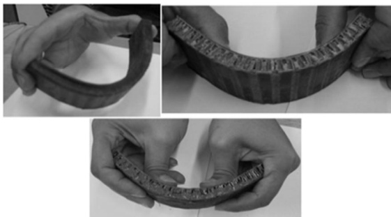
Fig. 2 Different flexibility of sandwich panel
