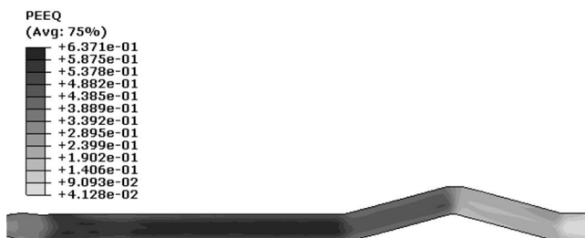
Fig 4 Deformed strips and equivalent plastic strain contour
