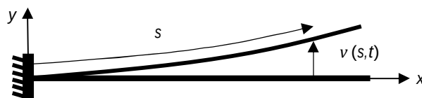
Fig. 1 Schematic of beam with large deflection
