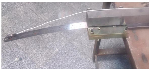
Fig. 8 Test set-up (beam with initial displacement)
