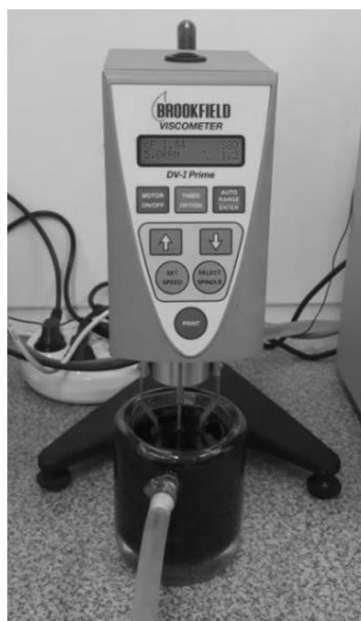
Fig. 2 Measurement of viscosity using Brookfield DV-I PRIME digital Viscometer equipped with a temperature bath
