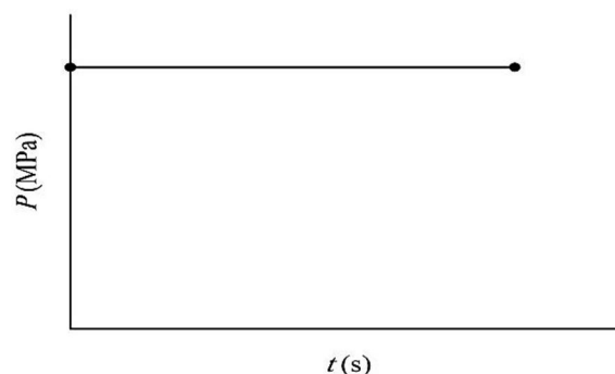
Fig. 6 Pressure path in tube multi-bulge test
