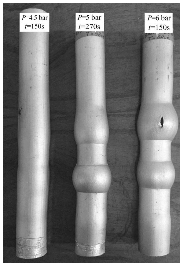
Fig. 21 The effect of pressure on the bulge height at 580°C
