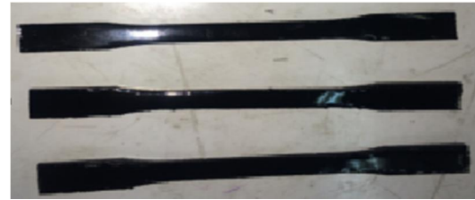
Fig.1 The tensile test specimens of the nano-resin
