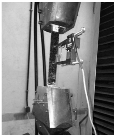
Fig. 3 The hybrid nanocomposite specimen under tensile test
