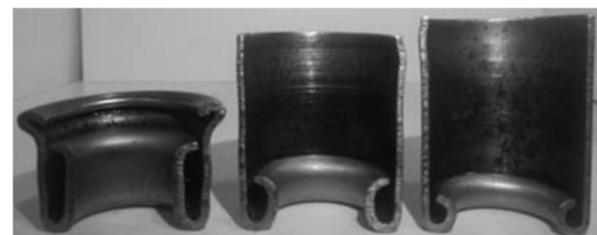
Fig. 18 Internally inverted sectioned tubes for the impact velocity of 89 m/s, (respectively from right to left, m=175 , 264 & 475 gr)
