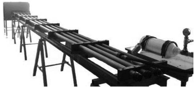
Fig. 1 Total view of Gas Gun
