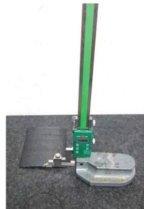
Fig.9 Measuring the displacement of the laminate by a height gauge
