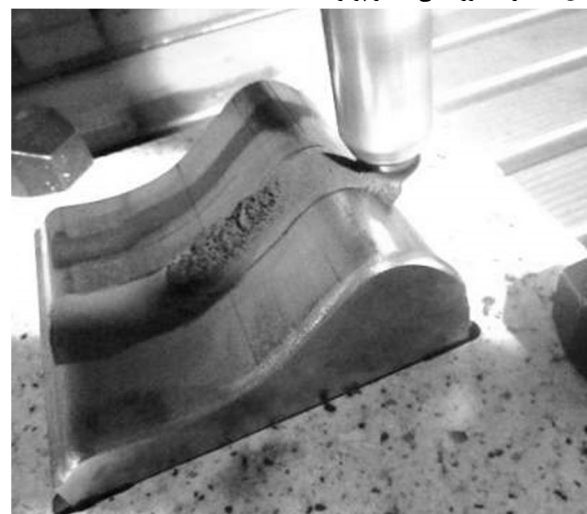
Fig. 25 remained powder on the work piece surface
