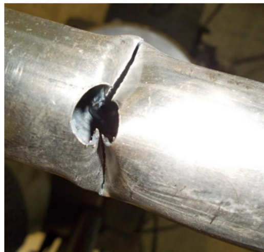
Fig.12 failure of specimen from location of cutout
