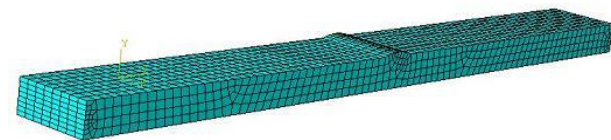
Fig. 8 Free meshing with linear tetrahedral and hexahedra elements
