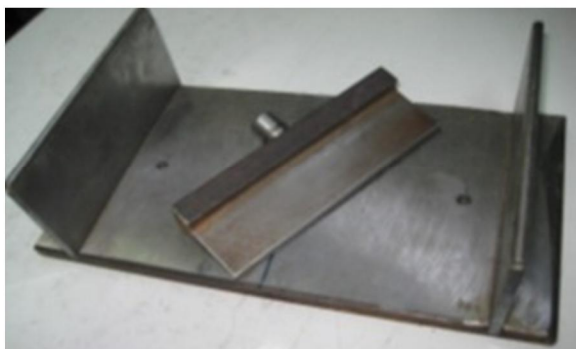
Fig. 6 Fixture of three-point bending
