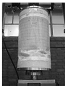
Fig. 7 Cylinder after buckling
