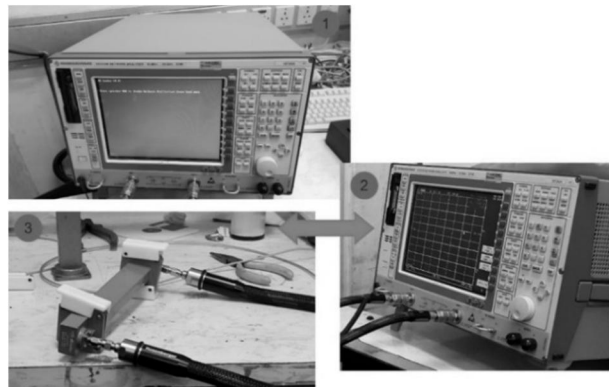
Fig. 11 1) Front view of Device 2) The device is ready for measurement 3) Putting samples in waveguide and measuring the amount of absorption
