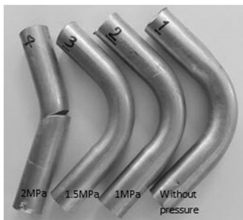
Fig. 11 Bent tubes in various pressures
