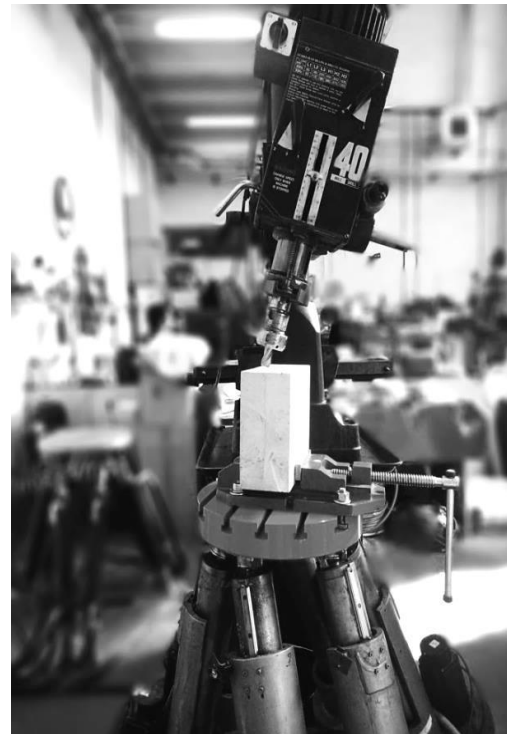
Fig. 2 Rotating the milling machine's head
