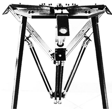
Fig.2 Manufactory model of the 3-[P2(US)] parallel manipulator
