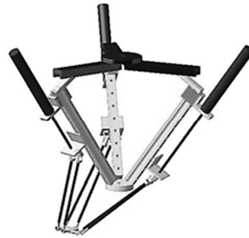
Fig. 1 Schematic of a 3[P2(US)] parallel manipulator
