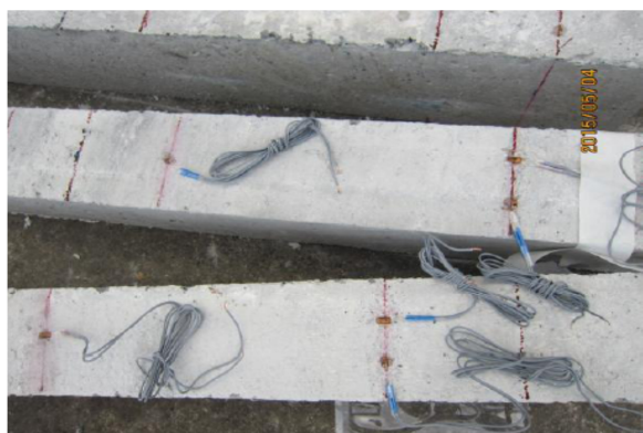
Fig. 11 Strain gauges attached to rubberized concrete
