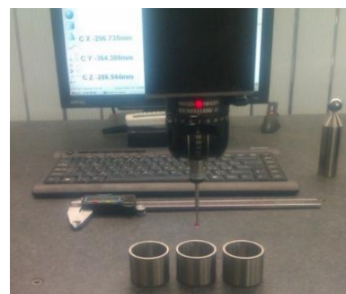
Fig. 2 Dimension measurement of the bush by Coordinate Measurement Machine (CMM)
