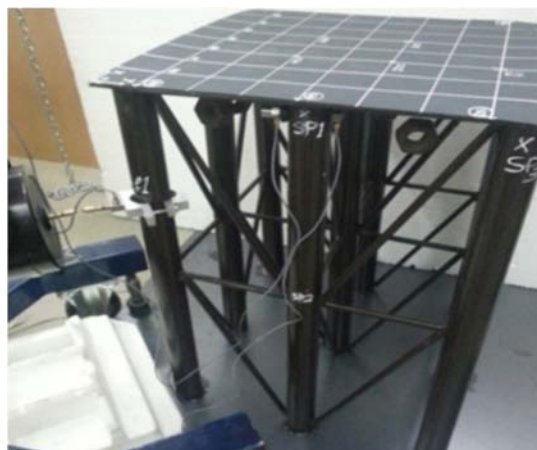
Fig. 1 The model of pier for experimental modal analysis
