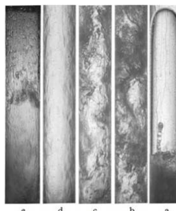
Fig. 6 Flow patterns in tube with inner diameter of 80 mm a) slug, b) churn, c) churn-annular, d) annular, e) reverse flow
