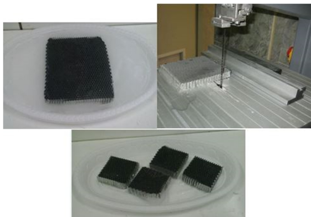
Fig.2 Preparation and cutting of honeycomb structures
