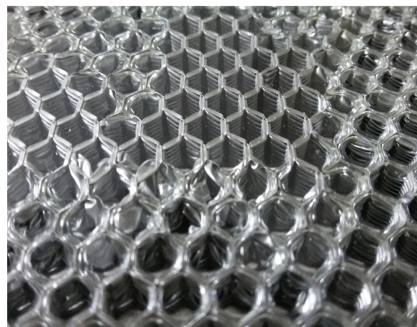
Fig. 7 empty sandwich panel core under distributed loading
