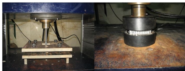
Fig. 4 Universal testing machine used in concentrated and distributed loading quasi-static tests
