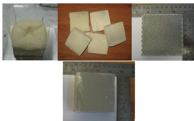
Fig. 3 Preparation of sandwich panels filled with foam
