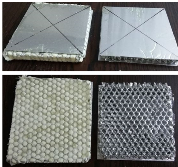
Fig. 6 empty and foam filled sandwich panel under distributed loading (from top to bottom, sandwich structures and sandwich panels without face sheet)
