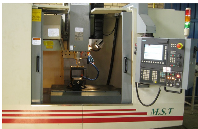
Fig. 9 Three axis CNC milling for incremental forming
