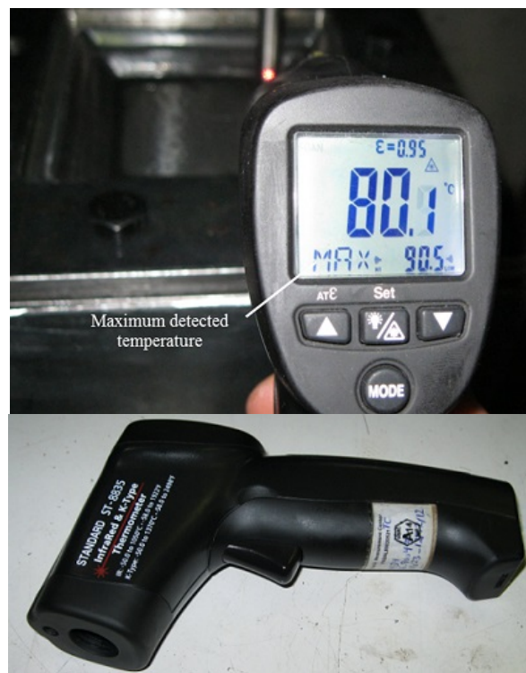
Fig. 11 Infrared thermometer to measure forming location temperature
