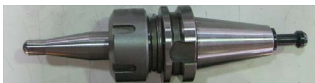
Fig. 7 hemispherical head tool with 9 mm diameter
