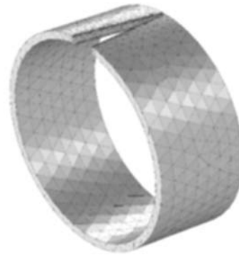
Fig.4 model meshed with tetrahedral element.
