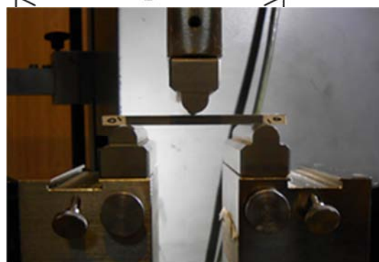
Fig. 6 Schematic and real view of fixture for the three-point bending test.
