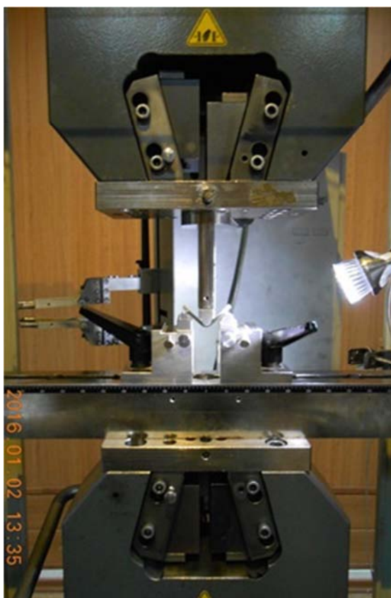
Fig. 8 The three-point bending test set-up.
