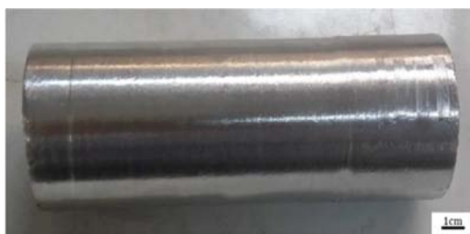
Fig. 3 Casting alloy sample after turning
