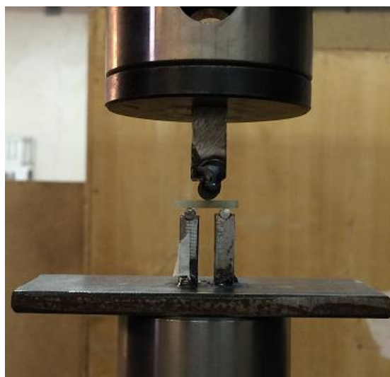
Fig. 2 Nanocomposites under short beam shear test
