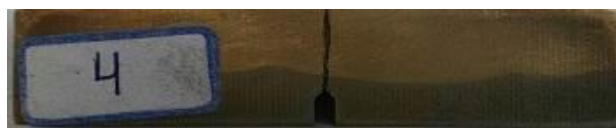
Fig. 4 A graded Copper-steel Specimen weakened by U-notch
