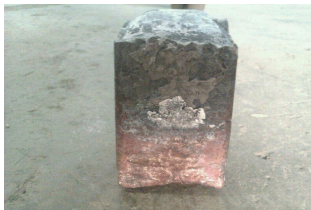
Fig. 3 Solidified copper-steel ingot
