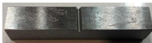
Fig. 8 Impact test sample according to ASTM E 23.
