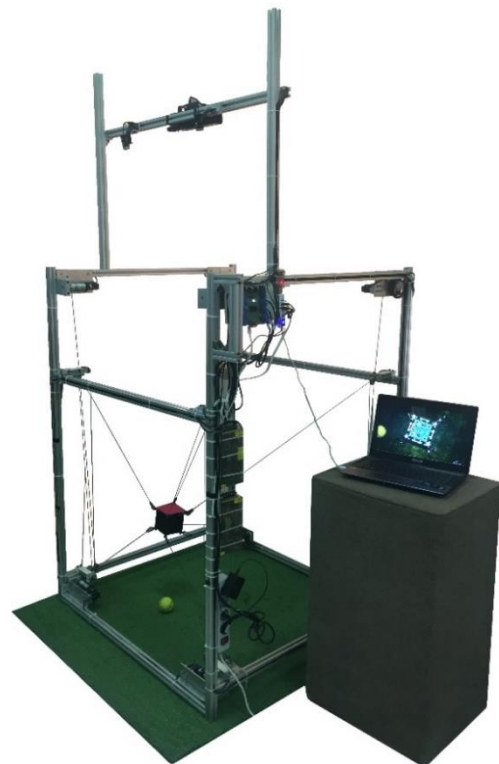
Fig. 1 6 DoF cable driven parallel robot, RoboCab
