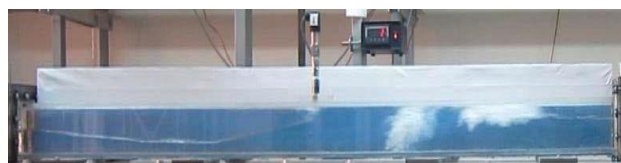
Fig. 2 Aerated slug flow in a duct [2]
