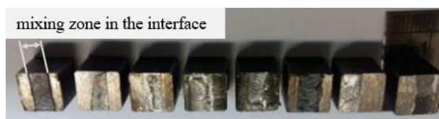
Fig. 12 Fracture surface samples tensile shear test
