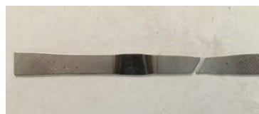
Fig.4 The fracture of base metal in uniaxial tensile test of friction stir welded specimen
