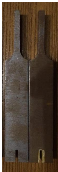
Fig.6 Fixtures made for fracture test
