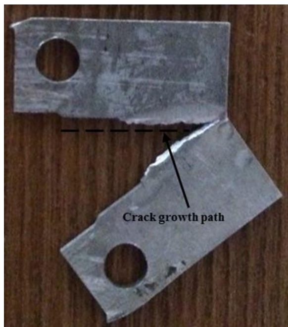
Fig.15 CT specimens after fracture test and crack growth path
