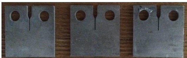
Fig.4 CT specimens before fracture test
