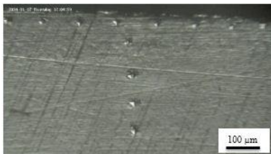
Fig. 10 Cross-sectional view of Vickers indenters in depth and surface of hardened zone
