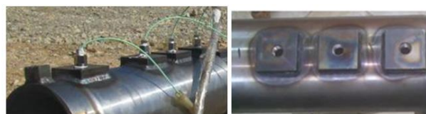
Fig. 3 test Sample and how to install pressure sensors
