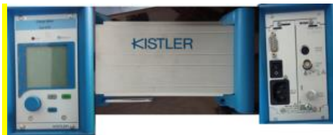
Fig. 7 Sample of device charging amplifier to boost signals
