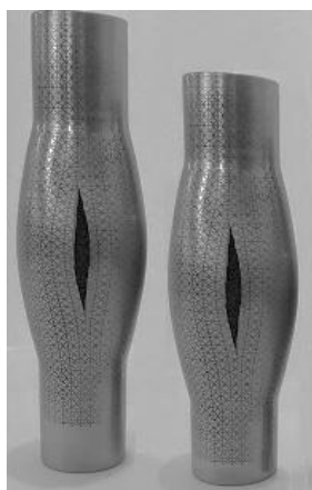
Fig. 20 A number of bulged components with various axial feeds (10mm, 5mm)
