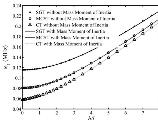
Fig. 2 Effect of the thickness to the material length scale ratio on the first flapping frequency of the rotating microbeam
