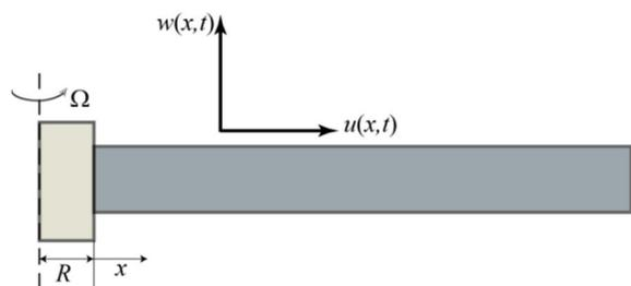
Fig. 1 A schematic of a rotating microbeam [29]
