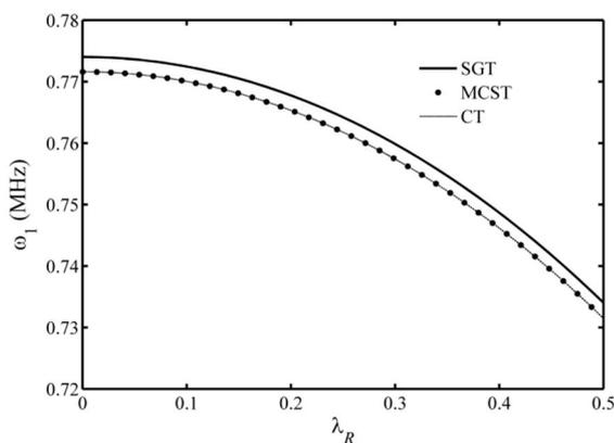
**Fig. 9** Effect of non-dimensional rotation speed of the microbeam on the first axial frequency
