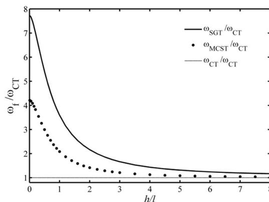
**Fig. 7** Effect of the thickness to the material length scale ratio on the ratio of the third flapping frequency predicted by strain gradient theory and modified couple stress theory to that calculated based on the classical theory of the rotating microbeam
