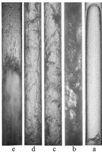
Fig. 3 Flow patterns in tube with inner diameter of 60 mm a) slug, b) churn-annular, d) annular, e) reverse flow
