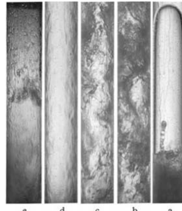
Fig. 6 Flow patterns in tube with inner diameter of 80 mm a) slug, b) churn, c) churn-annular, d) annular, e) reverse flow
