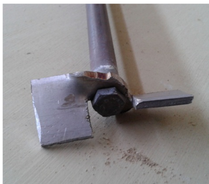
Fig. 3 View of stainless steel stirrer
