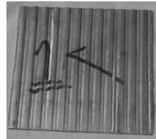
Fig. 5 The Al 5052 sheet fabricated by one pass of CGP
