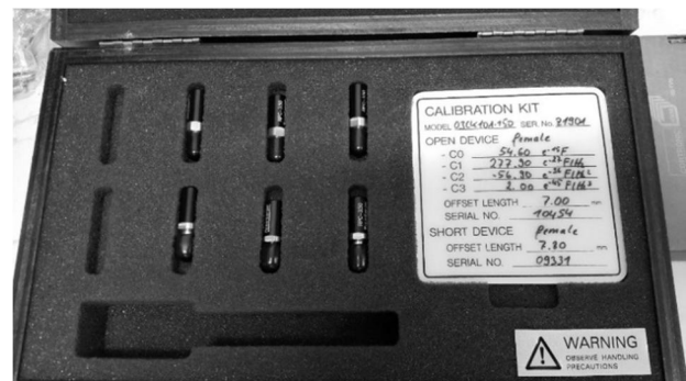
Fig. 8 A view of calibration tools in Math Load step
