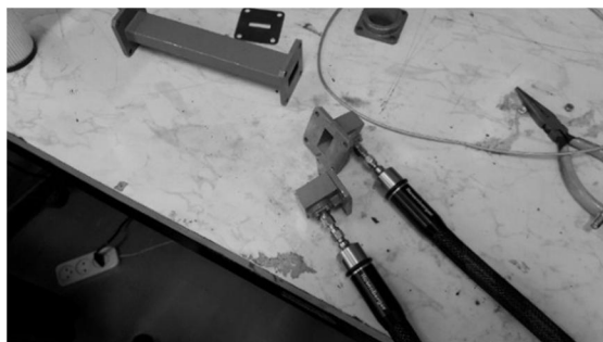
Fig. 9 A view of Short Load calibration step
