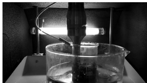
Fig. 3 Dispersion of SWCNTs in the Context of Acetone by Ultra-Sonic Mixer.
