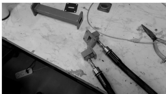
Fig. 9 A view of Short Load calibration step
