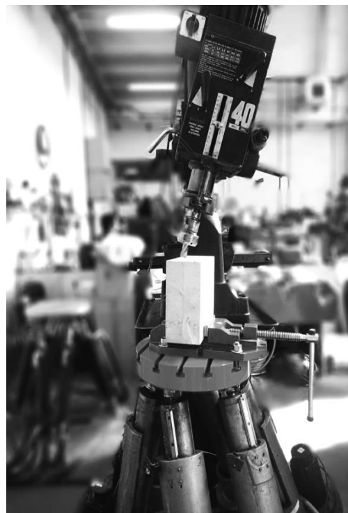
Fig. 2 Rotating the milling machine's head
